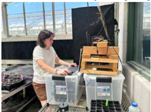
Figure 2. Miranda operates the homemade multispectral imaging device to estimate the anthocyanin and chlorophyll content of R. minus leaves.
